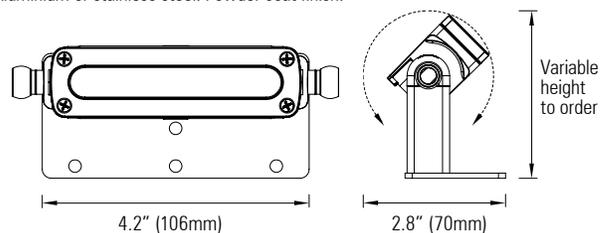
For adjustable-angle brackets, the angle of the modules can be adjusted by hand on-site
