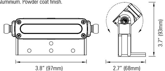
Custom height IP66 adjustable angle mounting bracket
