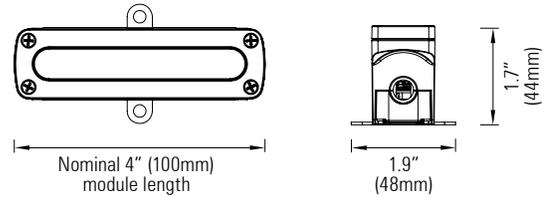
Backplate with raised mounting foot (fixed angle bracket)
